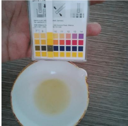
Figure 4. pH test of avocado leaf extract cream
