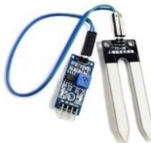
Gambar 4. Sensor Kelembaban YL-69
